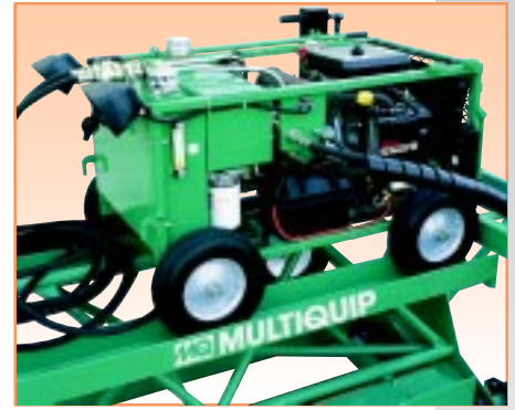
A powerful 20-HP Onan gasoline power pack ensures smooth performance.
