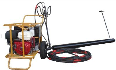
Juda Roller Screeds are 2500 powered by а psi Hydraulic Power Unit. Spinning at speeds up to 180 RPM in the opposite direction of travel, the Roller Tube strikes off concrete and moves the excess concrete forward.
